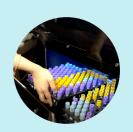
Robotic tube labelling Robot NESLİ labels and presents tubes directly to phlebotomist.
